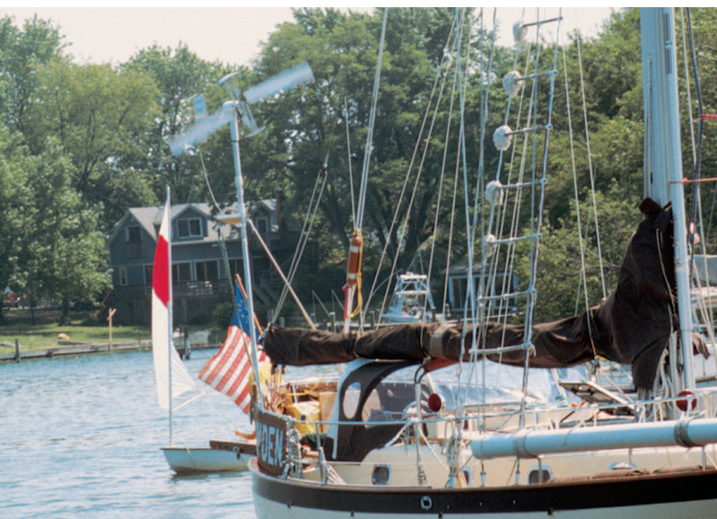
FIGURE 3.21 Wind is another form of solar energy. This wind turbine generates electrical energy for this sailboat, charging batteries for backup power when the wind is not blowing. In case you are wondering, the turbine cannot be used to make a wind to move the boat. In accord with Newton's laws of motion, this would not produce a net force on the boat. Source: © Bill W. Tillery.
